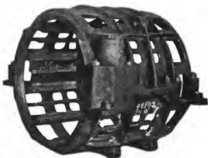
Fig. 4660. Skeleton Field Frame for Gearless Motor. Westinghouse A. C. Electric Locomotive.
